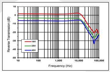
Figure 15: Magnitude of incremental reverse transmission (RT =  $i_m l_{out}$ ) for minimum, nominal, and maximum input voltage at full rated power.
