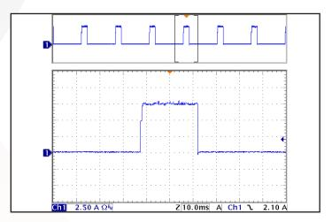
**Figure 18:** Load current (2.5A/div) as a function of time (10ms/div and 100ms/div) when the converter attempts to turn on into a 1 m $\Omega$  short circuit.
