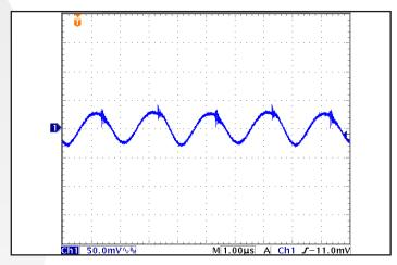
**Figure 10:** Output voltage ripple, Vout, at nominal input voltage and rated load current (50 mV/div). Load capacitance: 1μF ceramic capacitor and 15μF tantalum capacitor. Bandwidth: 20 MHz. Timescale: 1.00μs/div. See Figure 17.
