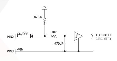
Figure B: Internal ON/OFF pin circuitry
