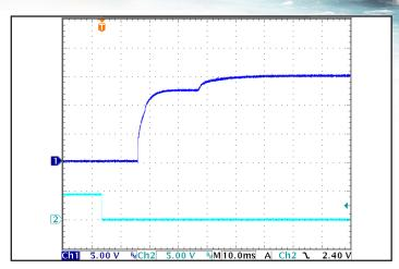
Figure 8: Typical startup waveform. Input voltage pre-applied. Ch 1: Vout (5V/div). Ch 2: ON/OFF Pin (5V/div). Timescale: 10.0ms/div.
