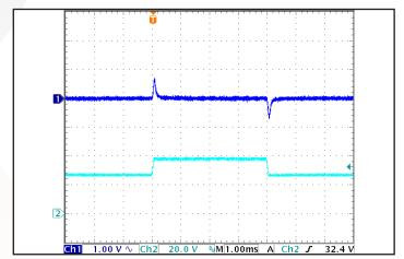
Figure 12: Output voltage response to step-change in input voltage (250V/ms). Load cap: 1uF ceramic and 15uF tantalum capacitance. Ch 1: Vout (1V/div), Ch 4: Vin (20V/div). Timescale: 1.00ms/div.
