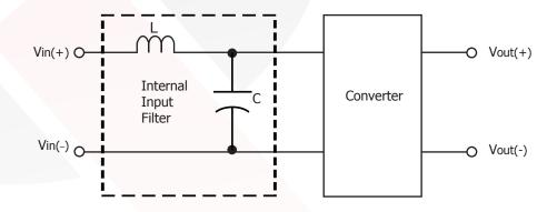
Figure E: Internal Input Filter Diagram
