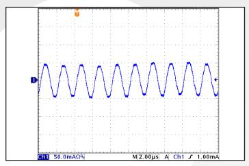
Figure 9: Input terminal current ripple,  $i_{c}$  at full rated output current and nominal input voltage with SynQor MCOTS filter module (50 mA/div). Bandwidth: 20 MHz. Timescale: 2.00 $\mu$ s/div. See Figure 17.
