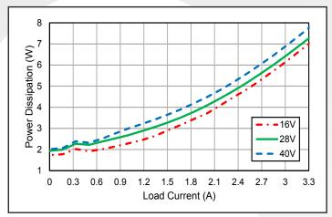
Figure 3: Power dissipation at nominal output voltage vs. load current for minimum, nominal, and maximum input voltage at T<sub>c.ss</sub>=25°C.
